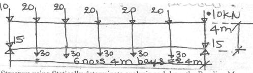
Analyse the Structure using Statically determinate analysis and draw the Bending Moment diagram.
