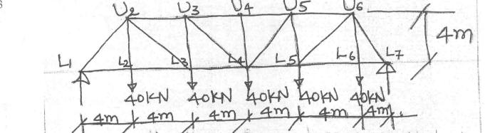
Determine the forces in members L<sub>1</sub>U<sub>2</sub>, U<sub>2</sub>L<sub>2</sub>, U<sub>3</sub>U<sub>3</sub>, L<sub>2</sub>L<sub>3</sub> & U<sub>3</sub>L<sub>3</sub> using method of Sections.
