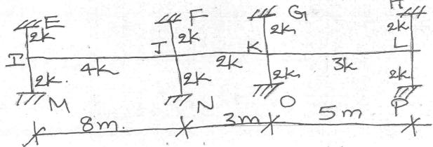
Total dead load = 25kN/m, 23kN/m & 24kN/m on spans IJ, JK & KL respectively. LL = 20kN/m on all spans.
